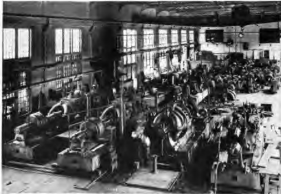
Testing Westinghouse-Parsons Steam Turbines
